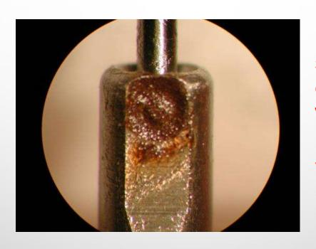
Moog flapper showing electrokinetic wear.
