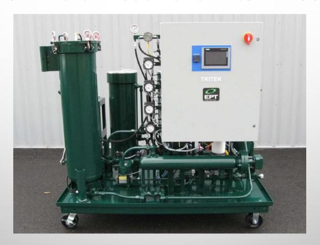
Two ICB IX cartridges, two ECR™ electrostatic collectors, a 6" x 18" 3 micron filter, TMR™ N2 (dry nitrogen) unit and heater.
