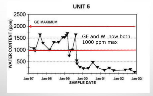
Dryer fluid can extend fluid life and also that of some purification media, and reduce maintenance on desiccant breathers.
