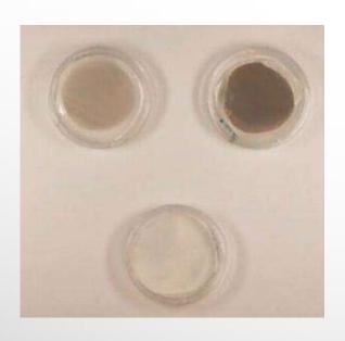
Note: The standard ASTM MPC test needs to be modified for phosphate ester fluids as does the reporting in some cases.
