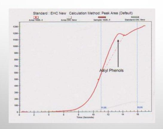
To large an area under the bump can indicate fluid degradation. Deposits and/or varnish can be more likely.
