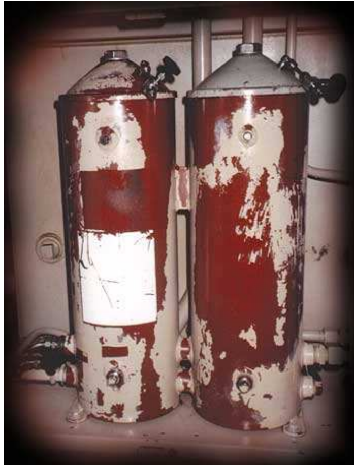
Figure 1. Purification Media Housing on an EHC System. Each Housing Takes One 718 Cartridge.
