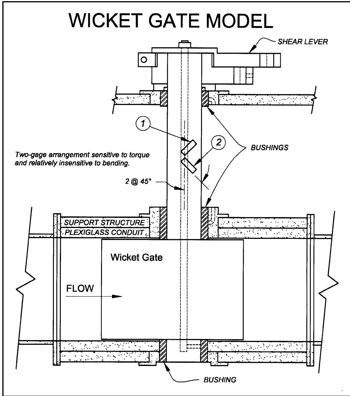
Figure 1.—Section through wicket gate model.
