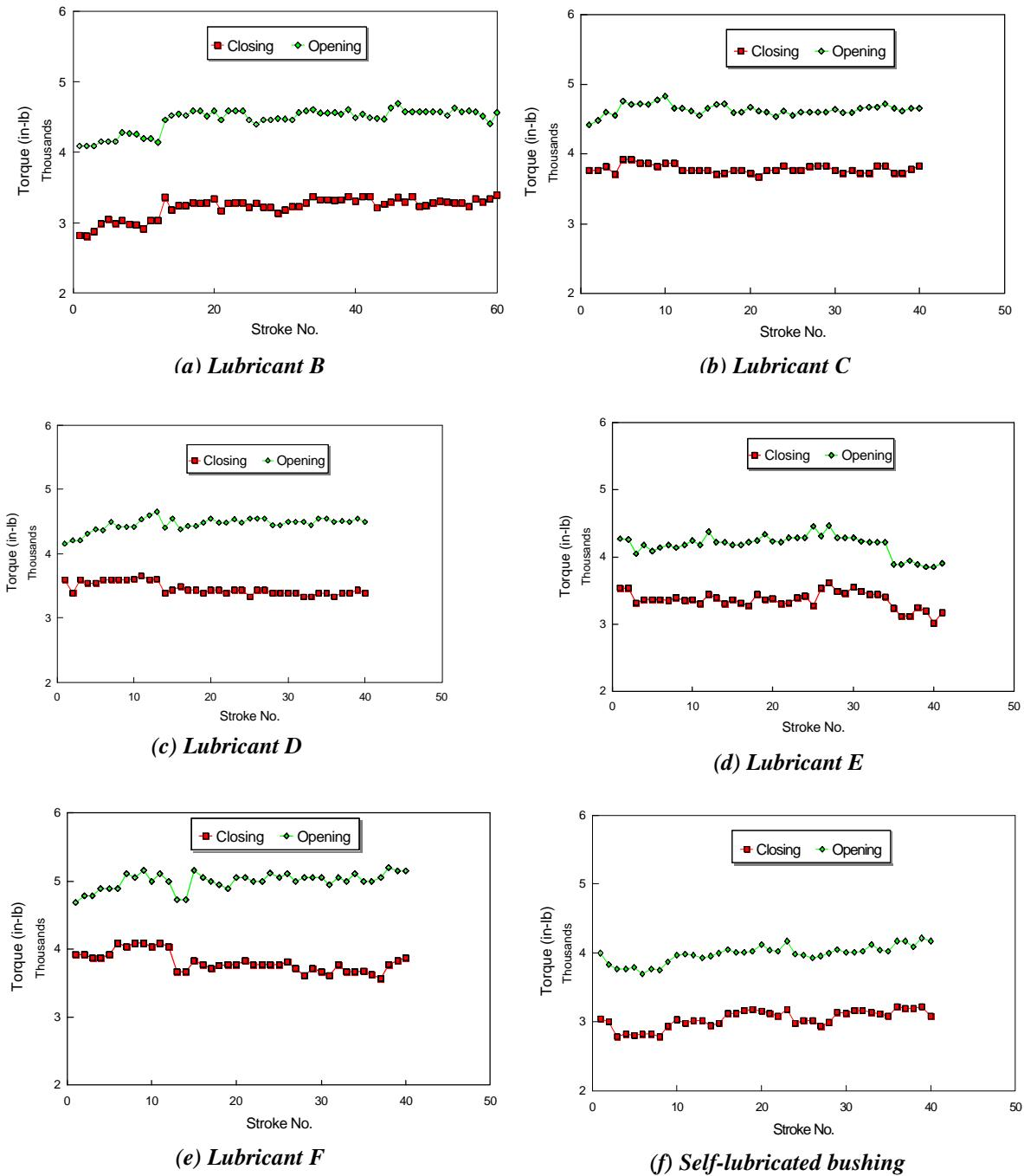
Figure 5.—Maximum torque versus stroke for five "green" lubricants and one self-lubricated bushing.
