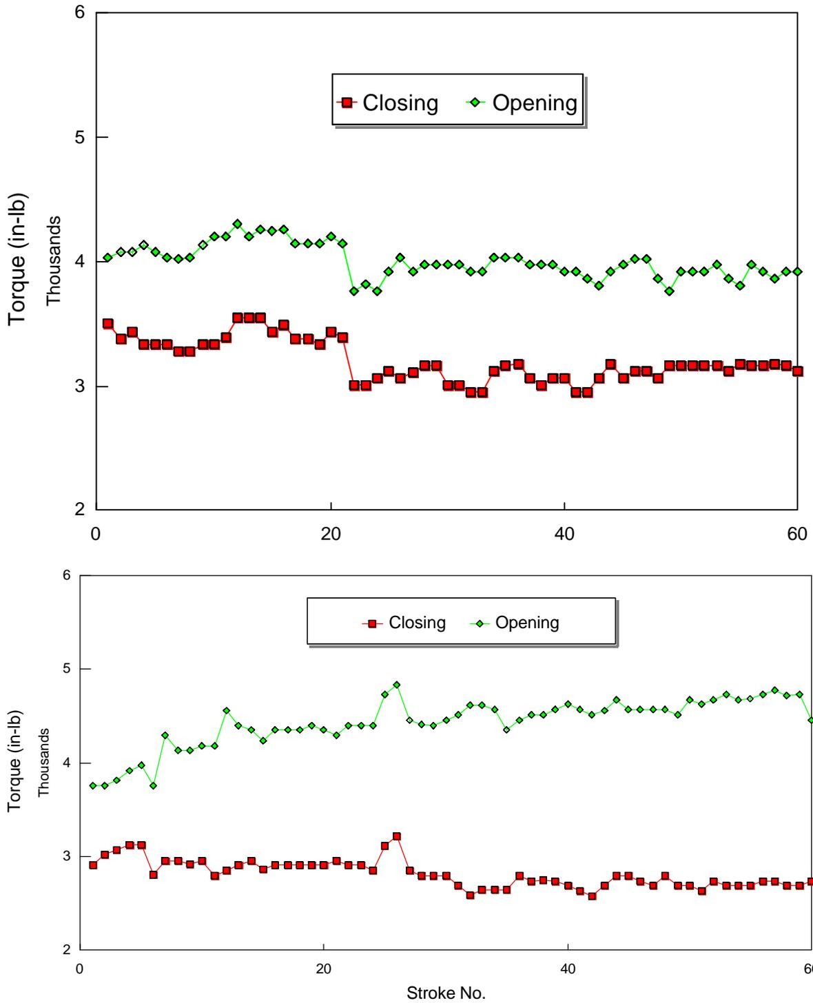
Figure 4.—Maximum torque versus stroke for baseline grease (above) and no grease—water only (below).
