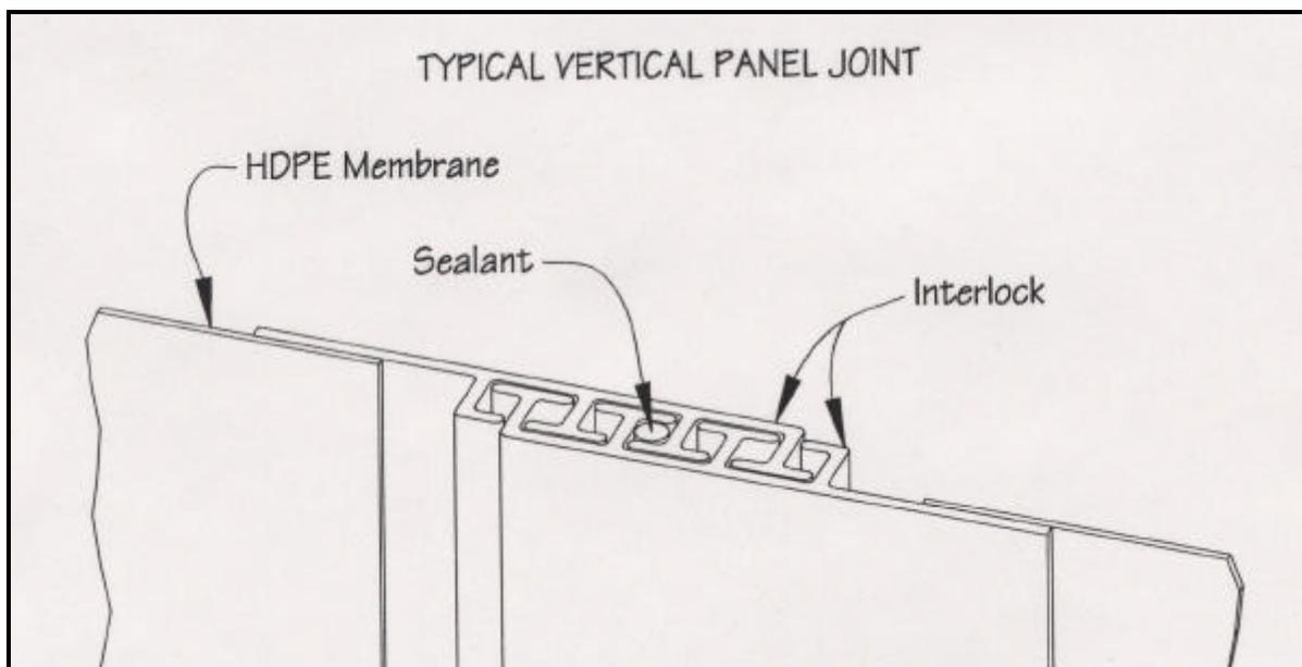
*Figure 1.—Placement of sealant in interlocked joint.*
