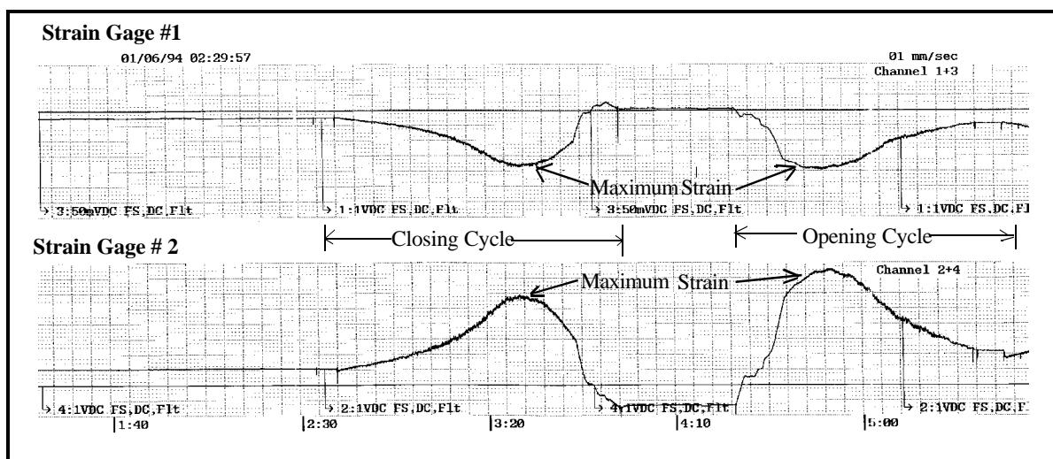
**Figure 3.—Typical recording of wicket gate closing and opening cycle.**
