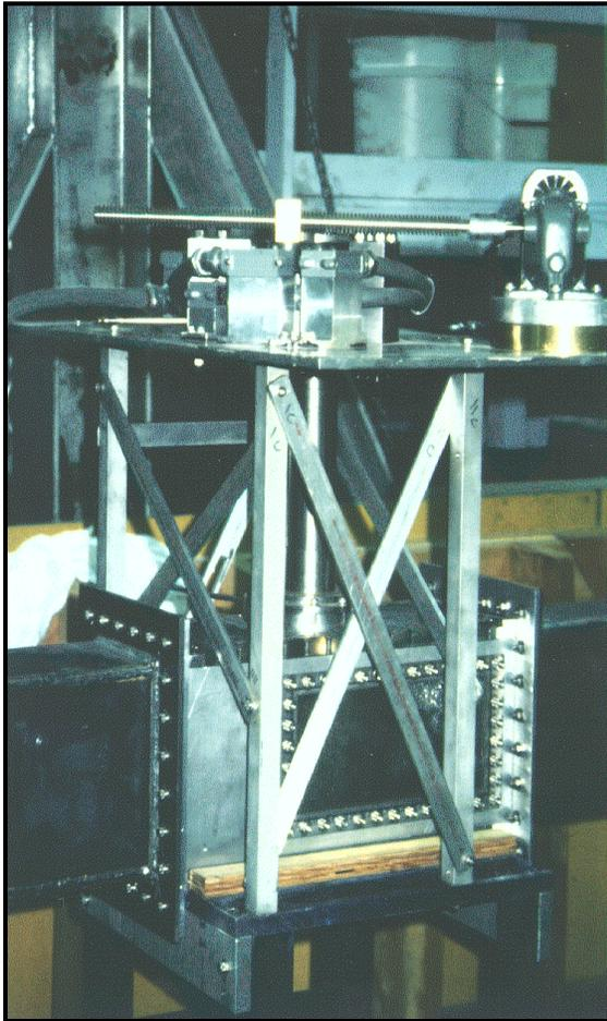
Figure 2.—Photograph of the wicket gate test apparatus.
