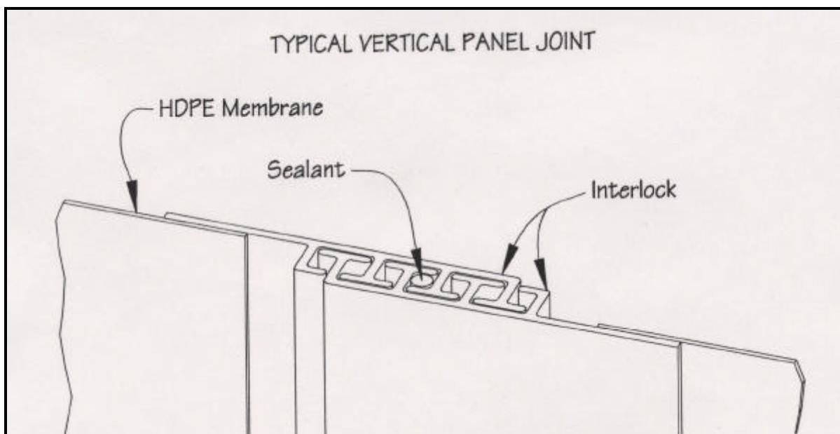
Figure 1.—Placement of sealant in interlocked joint.
