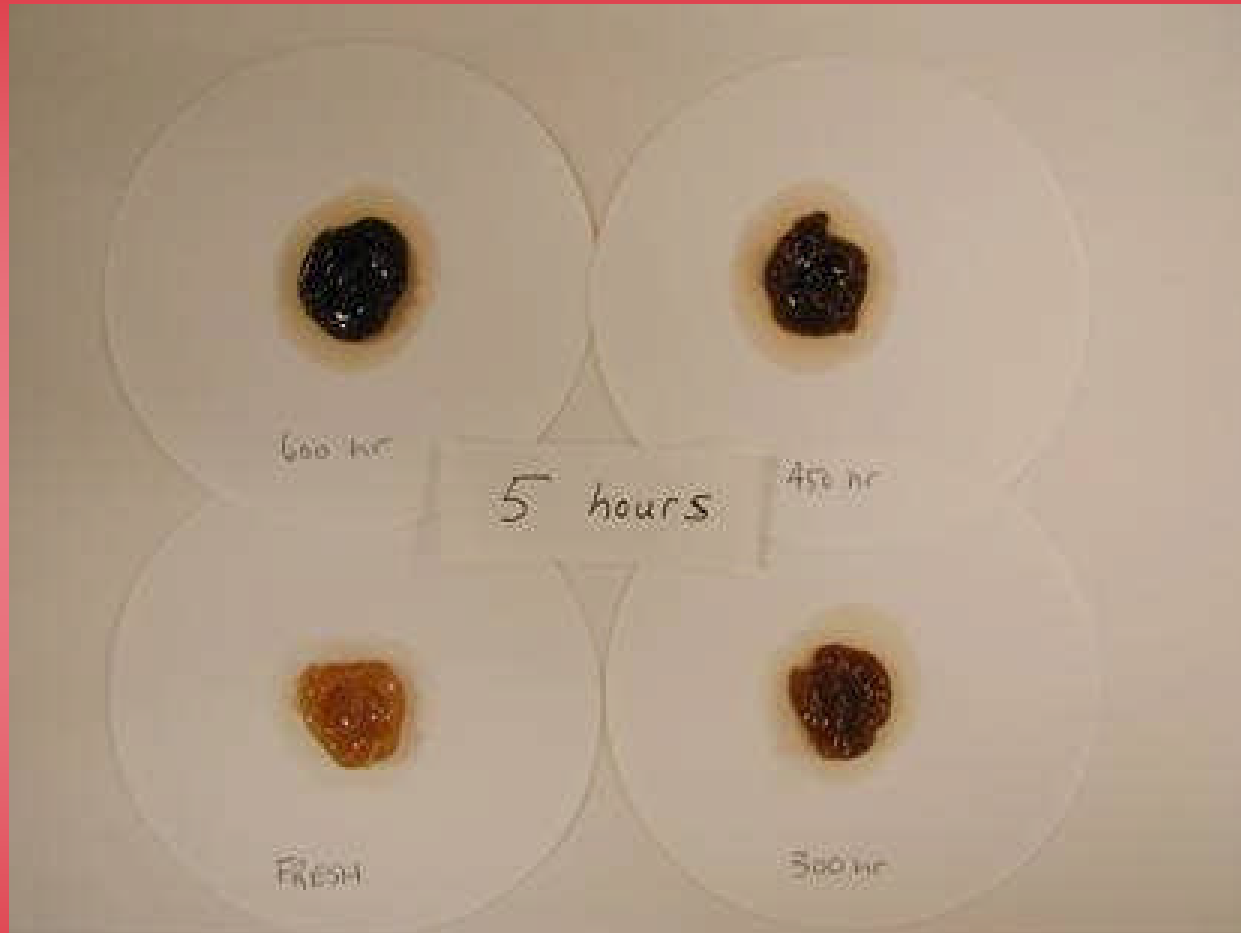
Fresh And Three Aged Samples – Color Change (Left For 5 Hours At Room Temperature)
